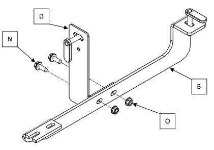
In the rear location install driver rear bracket (J) by first installing the bolt (L), washer (Q), and tab nut (M) into the driver rear bracket and then install into the hole towards the outside of the vehicle. Then install the bolt (N) through the backside of the vehicle and then through the bracket then put a nut (O) on the bolt. <u>Fully tighten hardware by pulling down on the bracket and tightening bolts.</u>
