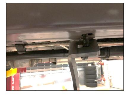
Next install the driver front support bracket (D) using bolt (L) washer (Q), and tab nut (M) into the front hole location. To tighten pull down on the brace and tighten bolt. <u>Do not fully tighten hardware at this time.</u>
