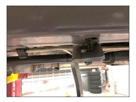
Next install the front support bracket (D) using bolt (I), washer (O), and tab nut (M) into the front hole location. To tighten pull down on the brace and tighten bolt. <u>Do not fully tighten hardware at this time.</u>
