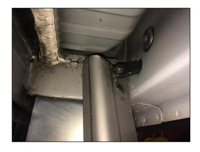
Connect driver rear bracket (J) and driver main bracket (F) by using bolts (S) and nuts (L). Fully tighten all hardware at this time.
