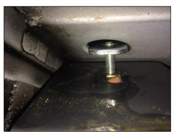
Install the bolt (I), washer (O) and tab nut (M) on driver rear bracket (J). Then install the tab nut into rear hole location. <u>Do not fully tighten hardware at this time.</u>
