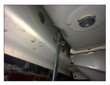
Connect The driver main front bracket (B) to the driver front support bracket (D) using bolts (N) and nuts (L). Fully tighten all hardware at this time.
