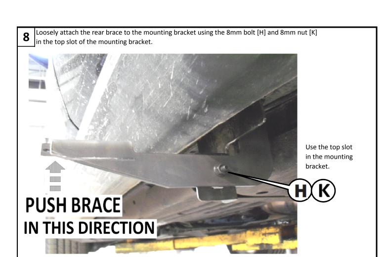
Push up on the rear brace to put tension on the bolt with the large threaded plate and tighten with a 13mm socket. Air tools are recomemded for this. Once the rear bolt has been tightened, tighten the bolt and nut attaching the brace to the mounting bracket using a 13mm socket and wrench.
