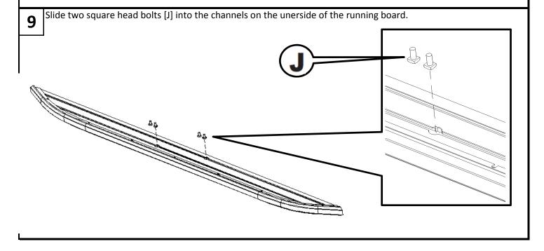
Line the bolts in the running board up with the slots in the braces.
