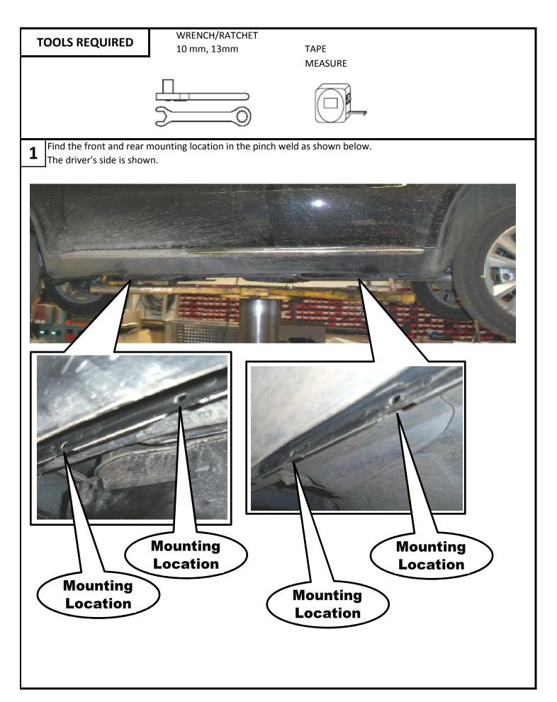
At each mounting location place a bolt plate into the holes in the pinch weld with the bolt studs pointing towards the outside of the vehicle.
