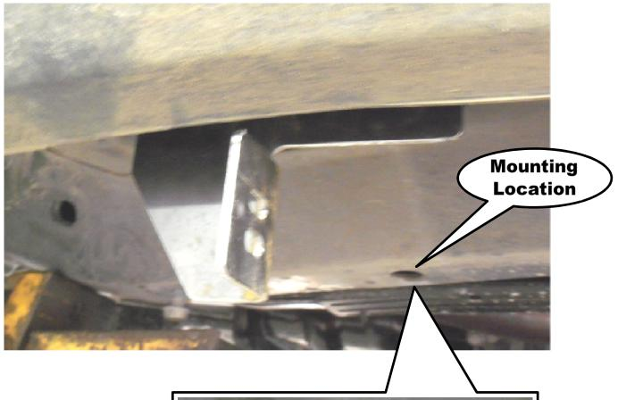
View from the front of the vehicle of the small threaded plate being installed.
