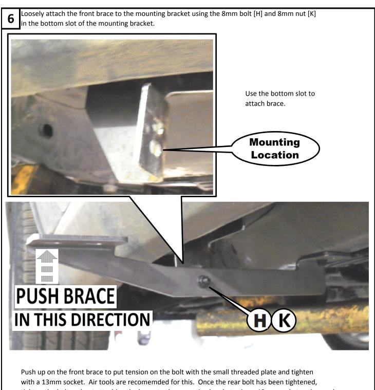
tighten the bolt and nut attaching the brace to the mounting bracket using a 13mm socket and wrench.
