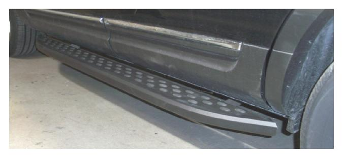
Attach the board to the braces using the flange nut [K]. Tighten all bolts with a 13mm socket.
