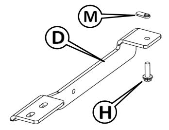
NOTE: Thread the bolt into the plate until the end of the bolt starts coming through the plate. Do not thread all the way through.
