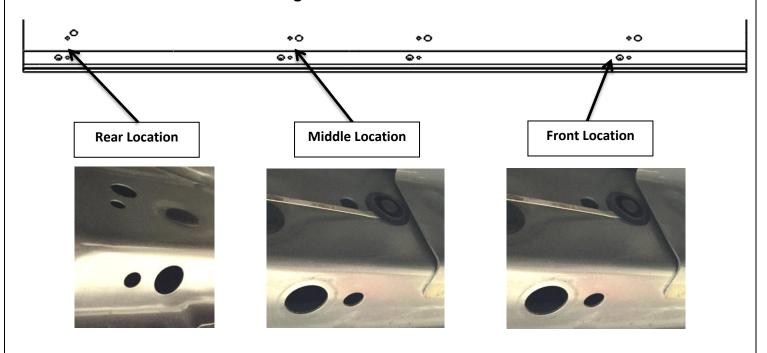
Install an 8mm U-nut (E) through each hole location that was covered by a plastic cap. To do this, insert the U-nut (E) into the hole and slide the U-nut (E) over so that the holes on the U-nut (E) and the vehicle are aligned, as illustrated below.
