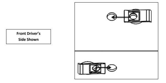
Attach a Right Bracket (C) to the Front Driver's Location, the Middle Passenger's Location, and the Rear Passenger's Location using two 8mm Hex Head Bolts (F) at each location. Do not completely tighten at this time.
