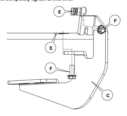
Attach a Left Bracket (D) to the Middle Driver's Location, the Rear Driver's Location, and the Front Passenger's Location using two 8mm Hex Head Bolts (F) at each location. Do not completely tighten at this time.
