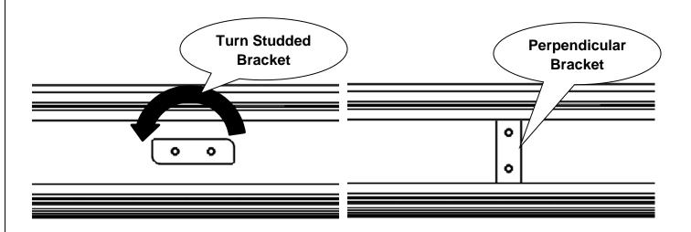
7b This Step is for installing the Molded Side Step ONLY. Go to step 5a for NXt Running Boards. Go to step 6a for Step Tubes.
