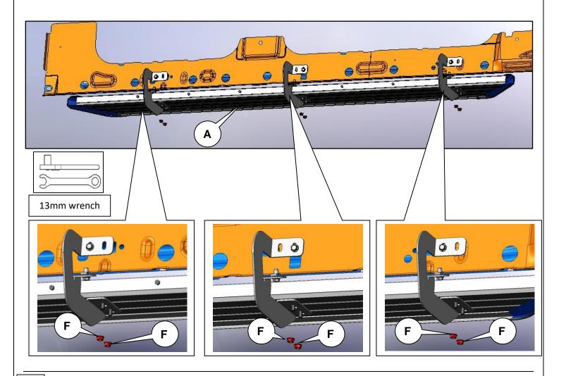
This step is for installing 6" Oval Step Tubes ONLY. Go to step 3 for NXt Running Boards. Go to step 5 for Molded Side Steps.
