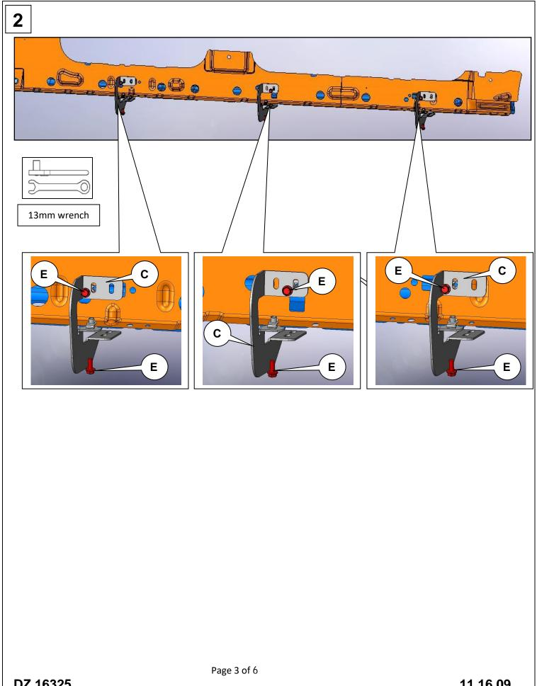
**DZ 16325** 11.16.09 This step is for installing NXt Running Boards ONLY. Go to step 4 for Step Tubes. Go to step 5 for Molded Side Steps.
