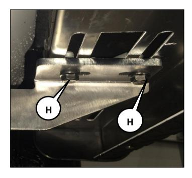
Once the tube is in the desired location, tighten hardware that connects the braces to the vehicle. Fully tighten all hardware at this time.
