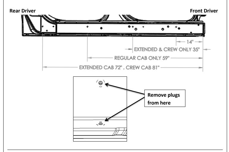
Attach a Bracket (C) to each of the Driver's side Locations where the plugs were removed in step 1 using two 8mm Hex Head Bolts (D) at each location. <u>Do not completely tighten at this time.</u>
