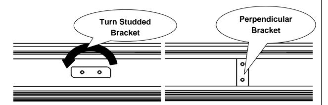
Install the board with studded brackets through the braces on the vehicle and install nuts on the studded brackets. Ensure Metal Framework of the board is touching the brace on both sides. Center the board front to back and Fully Tighten Hardware and repeat on the other side.
