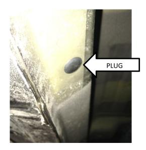
Use a standard screwdriver to lift the edge of the plug and a pair of pliers to pull the plug out.
