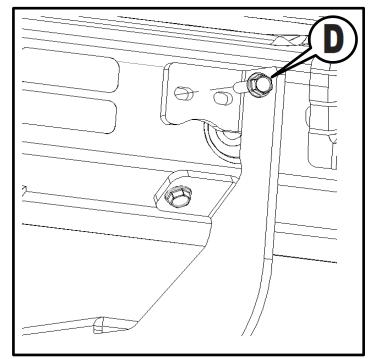
Tighten brace bolts with a 13mm socket / wrench.
