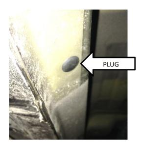
Use a standard screwdriver to lift the edge of the plug and a pair of pliers to pull the plug out.
