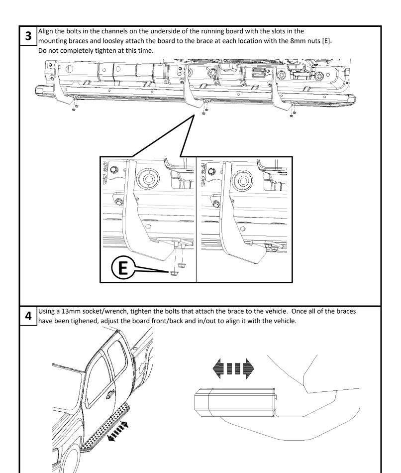
Once the board location has been set, tighten the nuts holding the board to the braces using a 13mm socket/wrench.
