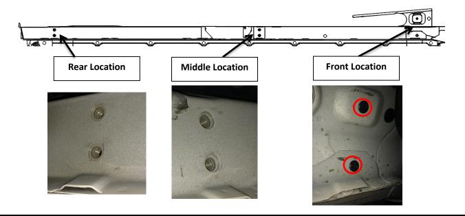
Attach the Left Front Bracket (C) to the Front Driver's Location using two 8mm Hex Head Bolts (G). Do not completely tighten at this time.
