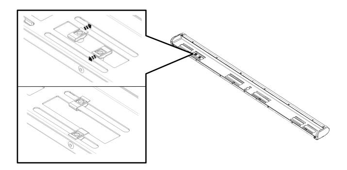
**5b** Tighten the Bolts (H) that connect the braces to the truck. Repeat for the other side.
