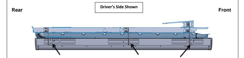
Remove the tube and install the 8mm U-nuts (J) that came with the Step Tubes (B) into the slots identified above. Use 2 U-nuts per brace location. Repeat on other side
