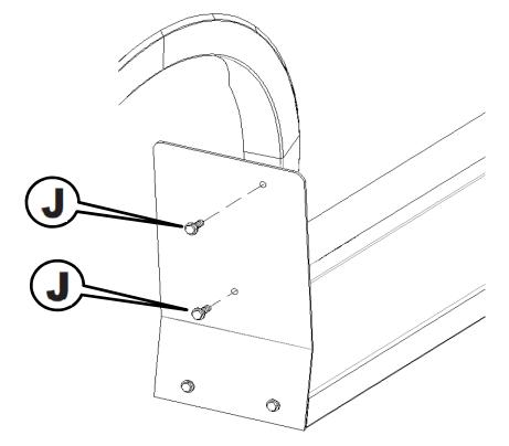
Check all hardware to make sure it has been tightened. Repeat the assembly steps for the other side of the vehicle.
