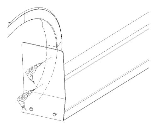
**12** Attach the mud flap to the wheel well using two sheet metal screws [K] with a 3/8" socket.
