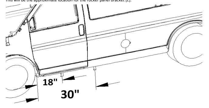
Make sure there is nothing on the bottom of the frame at these location that would obstruct the channel brace from being installed in the later steps. If there is an obstruction, move the rocker panel bracket to the front/rear as needed.
