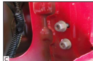
Inside the taillight opening, use an 11mm socket to remove the 2 nuts holding the rubber block in place.
