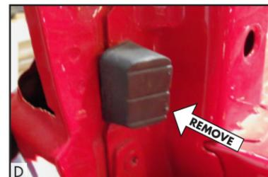
**WARNING: If the rubber block is not removed, it will interfere with the shock.**
