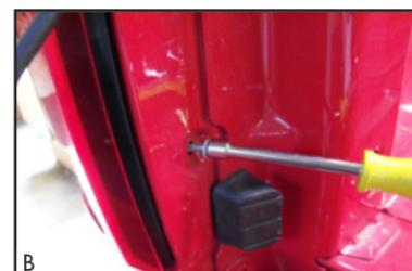
After removing the rubber block reinstall the taillight.
