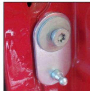
Tighten the bolt with the T50.
