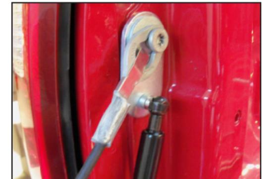
Install the narrow end of the shock on the ball mount.
