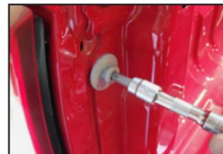
Install the bolt back through the hole in the ball mount into the vehicle.
