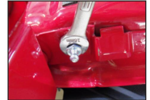
Using a torque wrench to install the ball mount will also insure that the blind nut has been completely installed.
