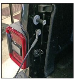
STEP 8 Reinstall bolts removed from step 1.
