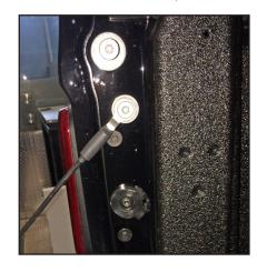
\*Periodically check the upper and lower mounting locations to insure that parts have not loosened through repeated use. If either mounting location is found to be loose, re-tighten the hardware as needed.
