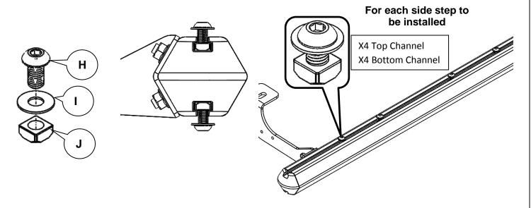
Install Side Step (F) by placing the side step(s) on the main tube (E) and sliding the button head bolts into the slots of the side step with the washer on top of the Side Step. Double check the placement of the side step by opening the door(s) then adjust as
