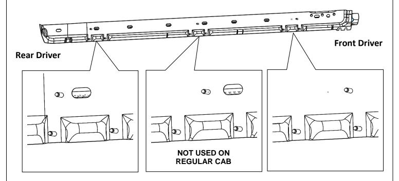
Use M8 Die (C) and a 26mm wrench to clean off paint from all of the studs. Ensure the die threads the entire length of the stud. <u>Failure to complete this step will result in a failure in the stud.</u>
