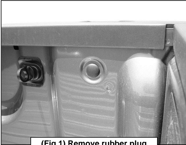
(Fig 1) Remove rubber plug from side of rear stake pocket
